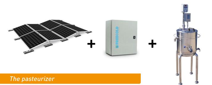
The FREECOLD<sup>®</sup> pasteurizer is designed for heat treatment of milk or juices with a capacity of 60 litres. Its electrical power limited to 2 KW, allows it to quickly heat a volume of milk at an adjustable temperature up to 95°C;
